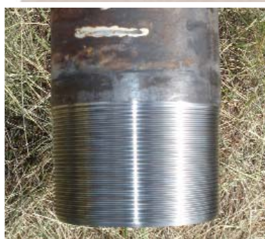
KORR-GUARD threads after over a year of storage on the Gulf Coast.
